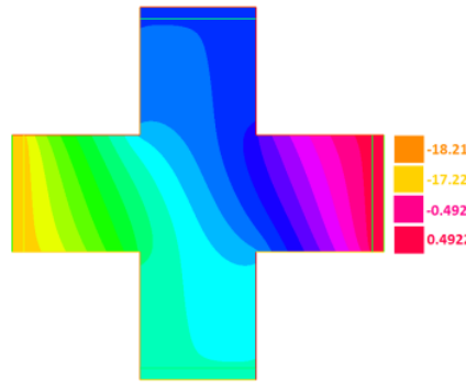
Figure 1: Simulated potential line distribution of a graphene Hall cross (1cm x 1cm) supplied with I = 1 mA under a B = 1 T magnetic field. Length/Channel Width, L/W = 3 .
